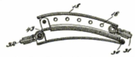
In an extension device for a wrist watch rality of sections hinged together to fold on one of said sections comprising two parts sl the other, means for retaining said sections i tion and at the same time preventing sliding one on the other whereby said sections must l slide the parts one on the other.
