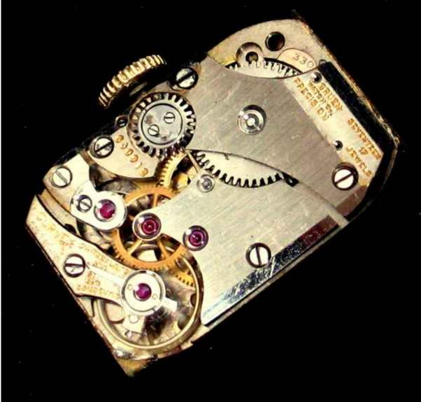
Subject: Re: The caliber 330 Posted by Thojil on Thu, 11 Jul 2013 11:55:06 GMT Interesting detail is that the 330 was initially produced with a single center bridge. Gruen changed to a split layout with separate escape wheel cock apparently in the fall of 1938 to improve serviceability (information I recall having from Cary).
