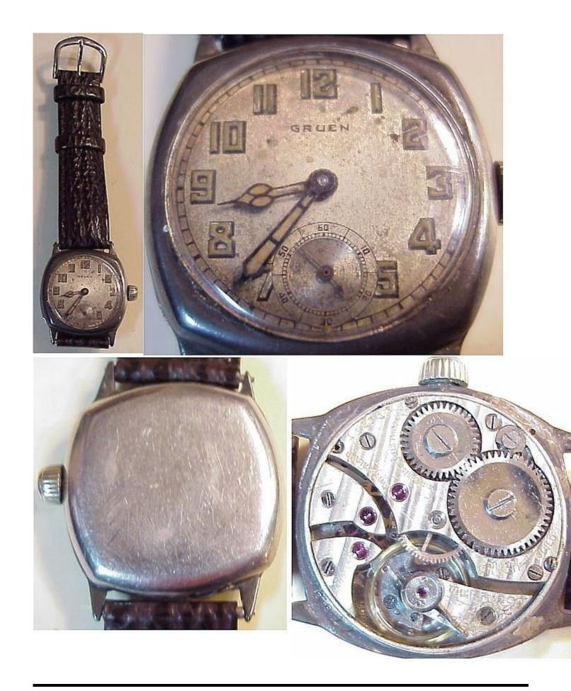
Do the presence or absence of case screw marks give any hints as to whether the center and bezel are original to the movement?
